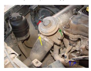
Remove 2 x 5mm Allen bolts securing the EGR valve re-circulation pipe to exhaust manifold. These are marked by red arrow in photo below.
