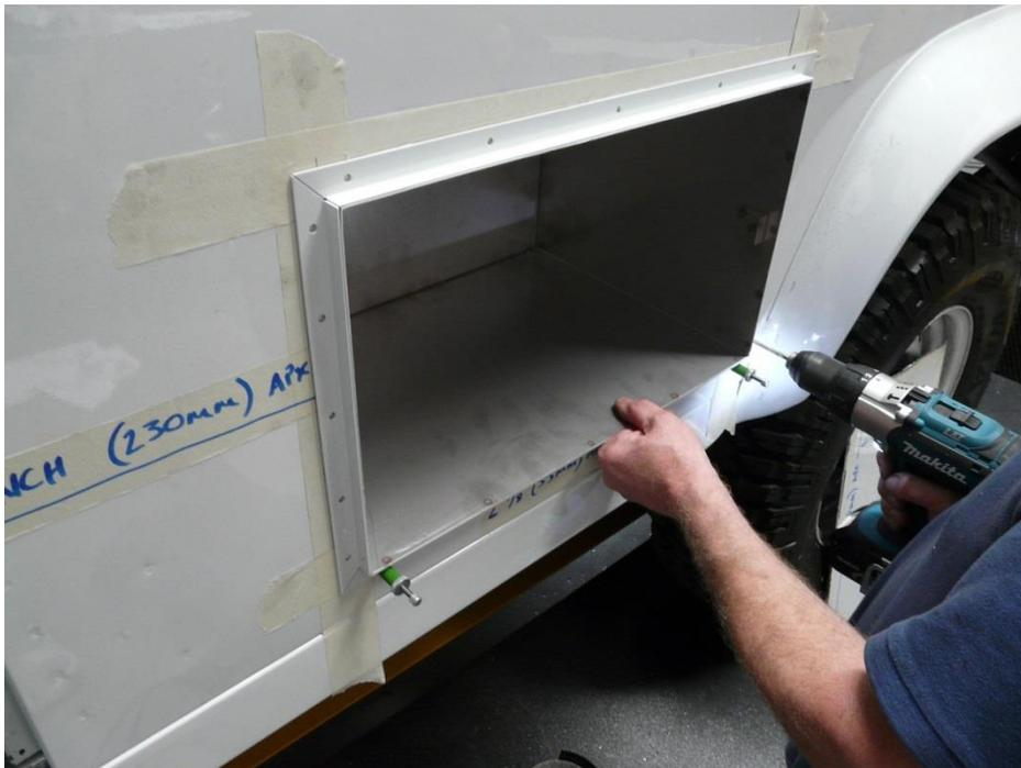
Some fitters like to use a small amount of bond between the mating surface's, should you wish to do the same please use a suitable bond compatible with all materials.
