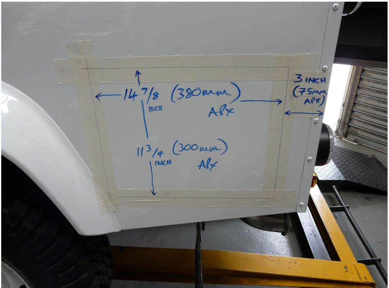
The key to fitting the rear locker is masking tape, a ruler, tape measure and a pen. You can accurately measure out where you want to cut the vehicle and check the box and cut lines for a tight fit and for square.
