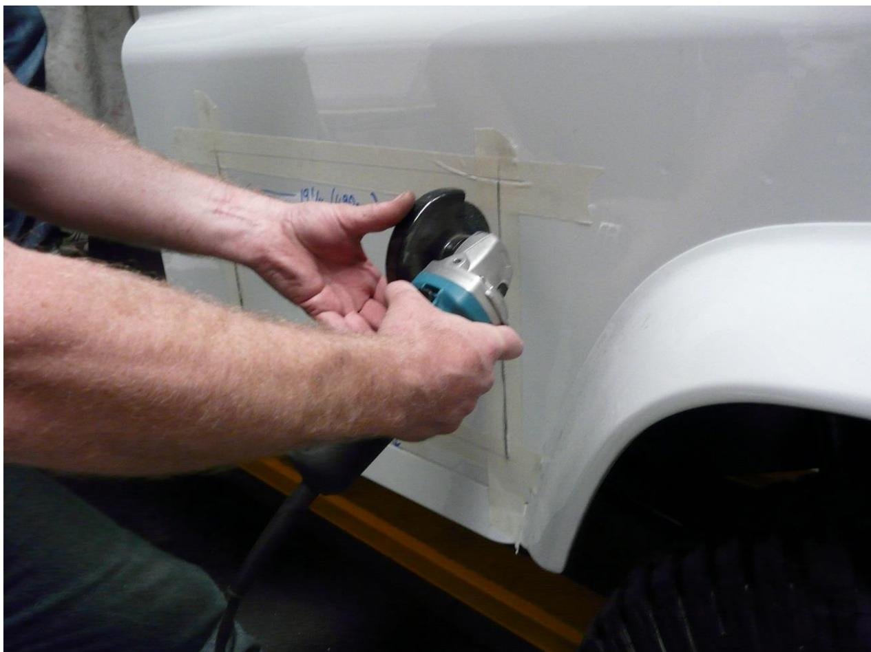
Once you have measured and checked, measured and checked again and you are happy an ultra-thin metal cutting disc is recommended, but take extra care at the corners and be careful of the heat generated.
