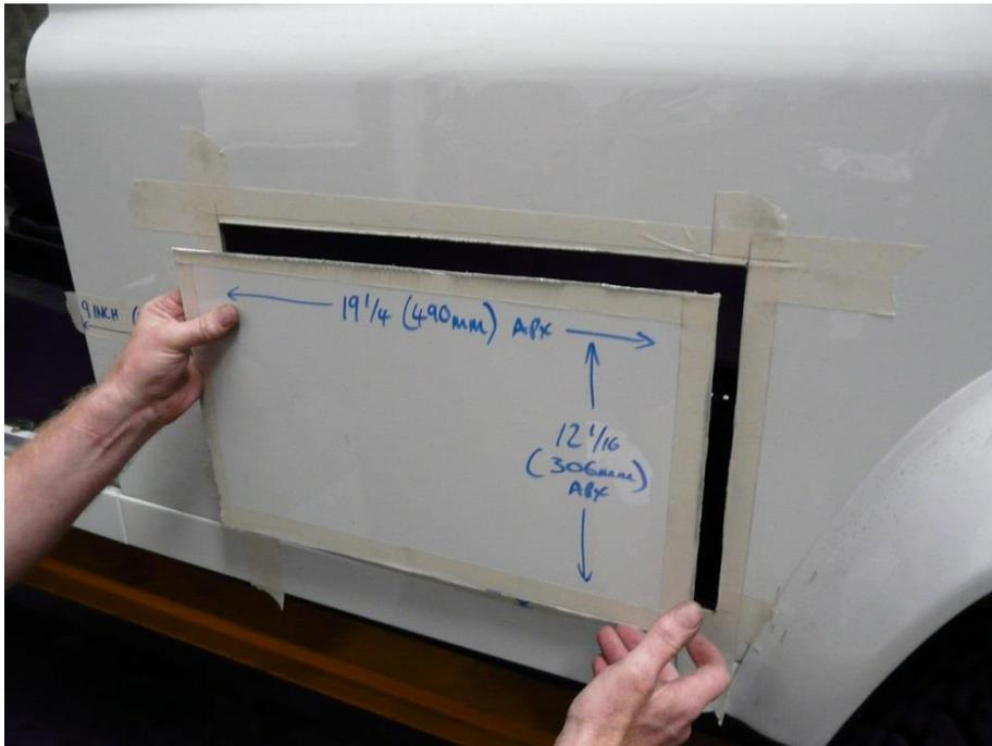
Once the area has been prepared for the locker then it should be fixed in place using the fastenings provided.
